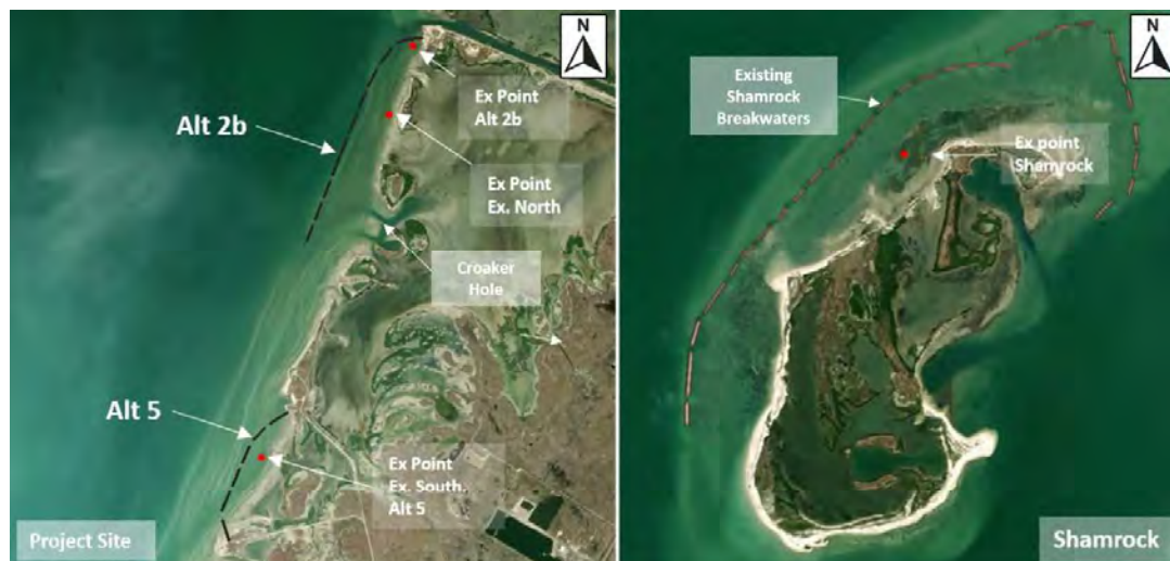
Figure 2-6. Final alternatives and extraction points used for comparative analysis. Ex point on Shamrock will be compared to Ex points on Alt 2b and Alt 5 to assure proposed alternatives will have similar hydrodynamic conditions conducive to sea grass growth, as is the case on Ex point Shamrock.
